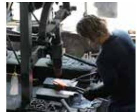
Thin and strong blades are brought to completion using the traditional forging technology of shaping with heat.
